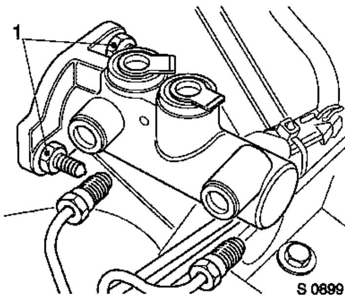
Blanking plugs from master cylinder and brake lines.
